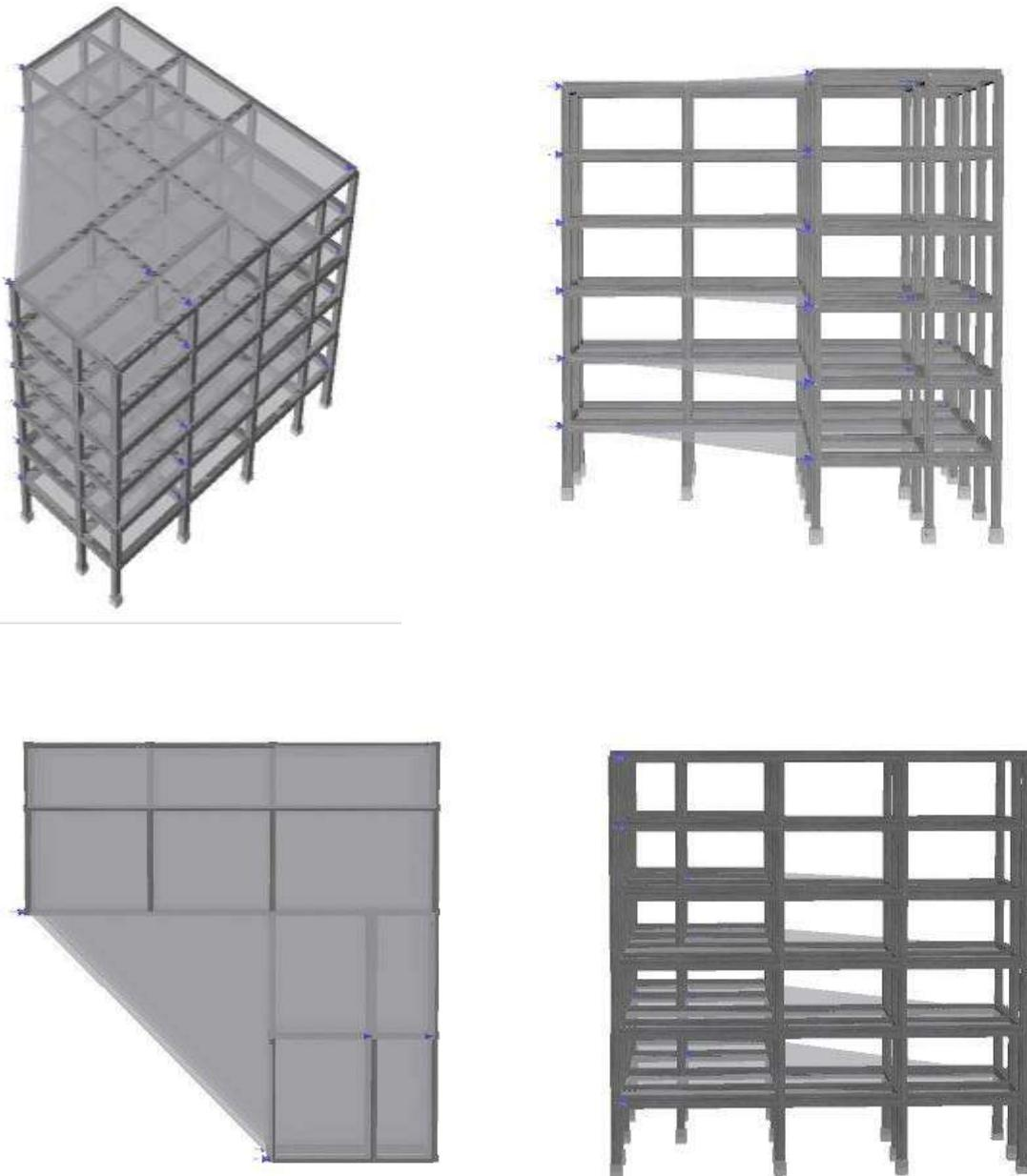
*Figure-1 6-Storey (inverted L-Shape) Seismostruct Model*
