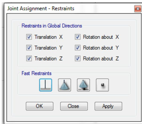
**Fig 3 Assigning support conditions**
