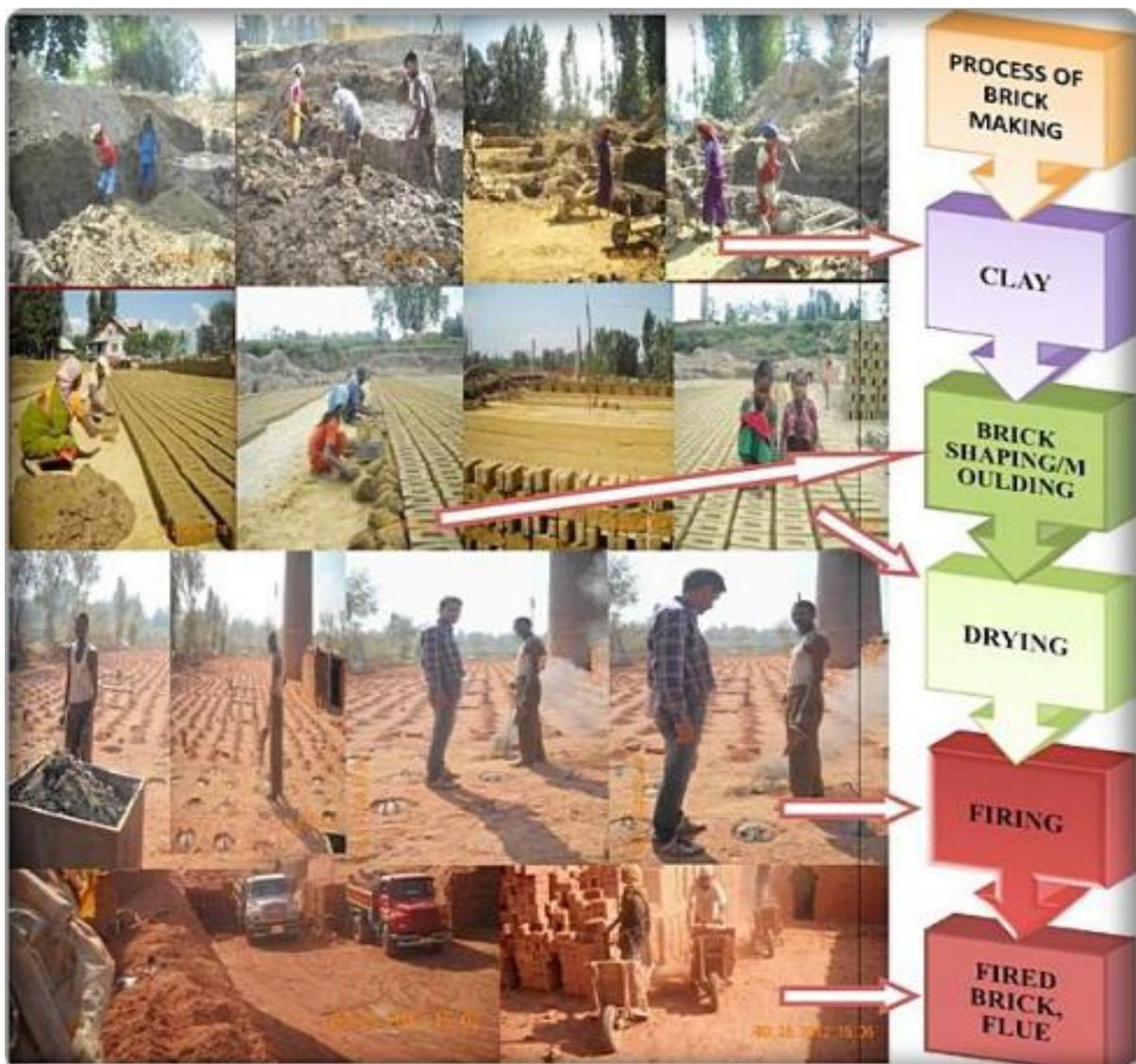
Process of clay brick manufacturing
