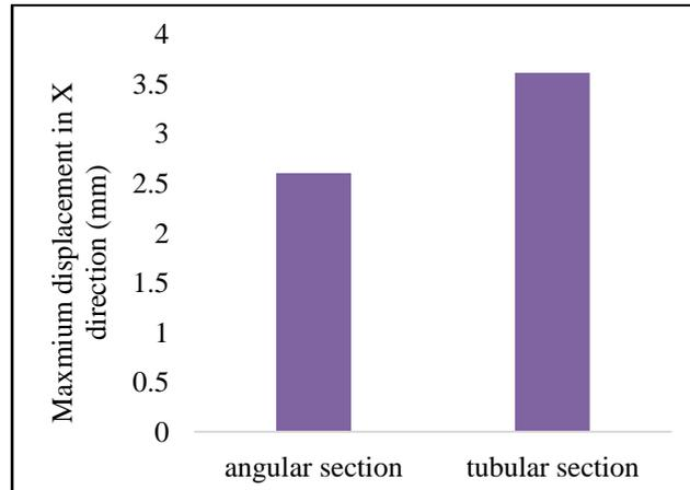
Fig. 13 Maximum displacement in tower with W bracing for different sections
