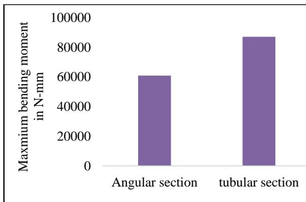
Fig.10 Maximum bending moment in tower with W bracing for different sections
