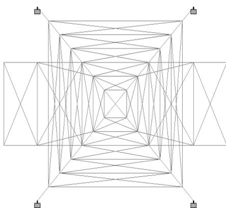
Fig. 1 Plan of the tower with X bracing
