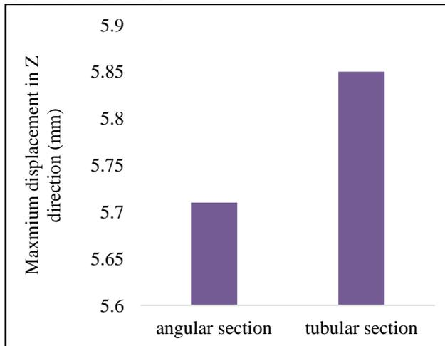
Fig. 14 Maximum displacement in tower with X bracing for different sections
