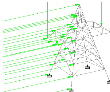
Fig. 7 Assigning of combination load
