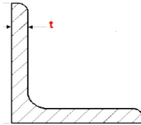
Fig. 3 Basic view of Angular section 200 mm X 200 mm X 25 mm
