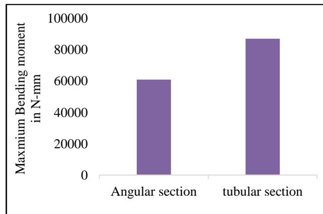
Fig. 9 Maximum bending moment in tower with X bracing for different sections
