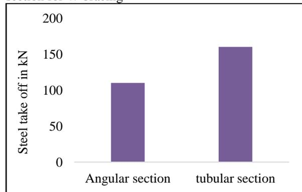
Fig.19 Steel take off comparison of angular and tubular section for X bracing
