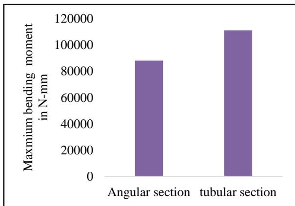
Fig. 8 Maximum bending moment in tower with K bracing for different sections
