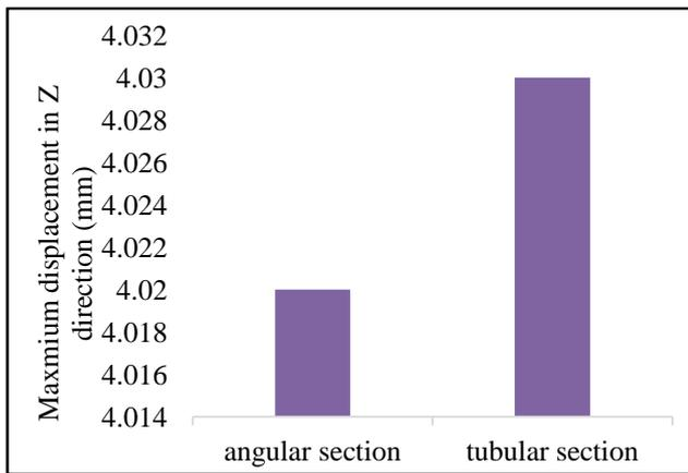
Fig. 16 Maximum displacement in tower with K bracing for different sections
