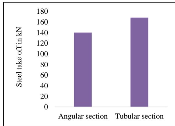
Fig. 17 Steel take off comparison of angular and tubular section for W bracing
