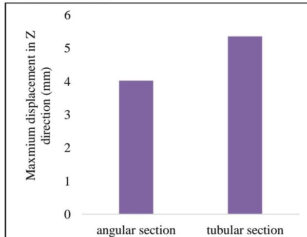
Fig. 15 Maximum displacement in tower with W bracing for different sections
