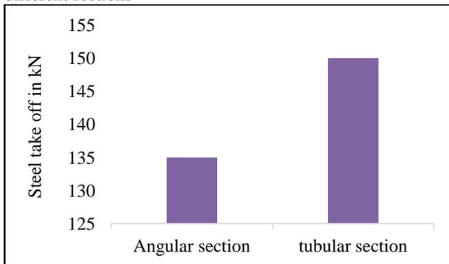
Fig.18 Steel take off comparison of angular and tubular section for K bracing
