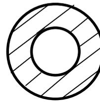
Fig. 4 Basic view of Tubular section 150mm diameter and 6 mm thickness
