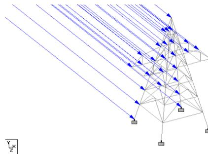
Fig. 6 Assigning Wind load in Z- Direction
