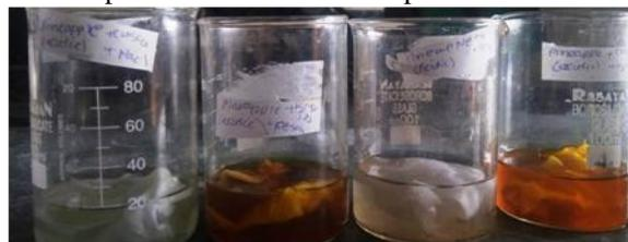
Fig 6 cotton cloth dipped in solvent containing different Mordant
