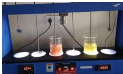
Fig 4 Pineapple mixture in flocculator
