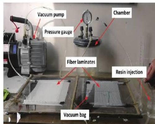
Fig: vacuum bag molding process
