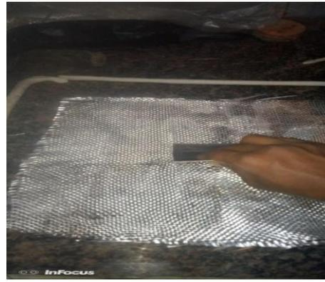
Fig: E-glass with resin
