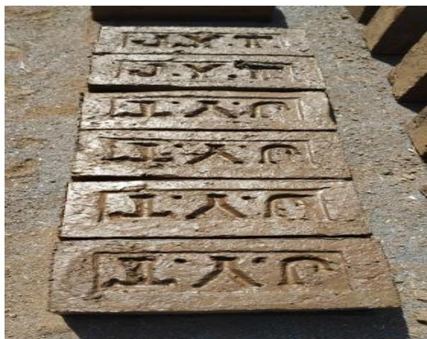
*Fig-1: Drying of RHA bricks*
