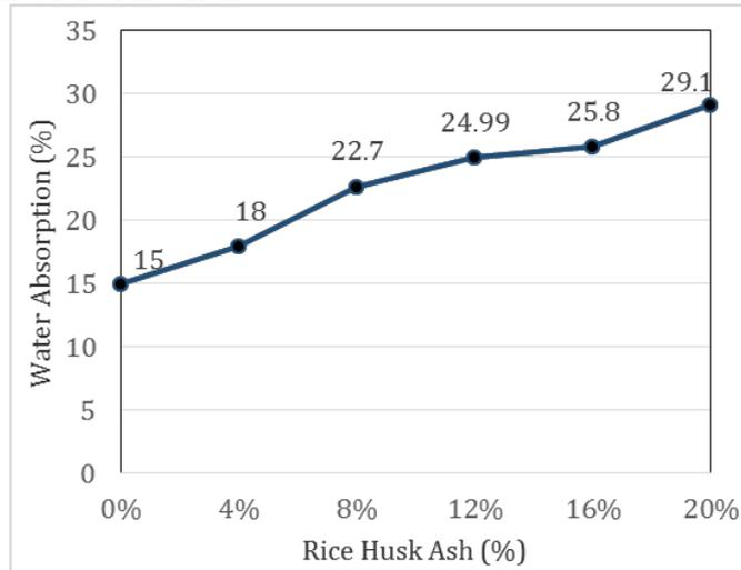
*Chart-2: Water Absorption of brick specimens with difference addition of Rice Husk Ash (%)*
