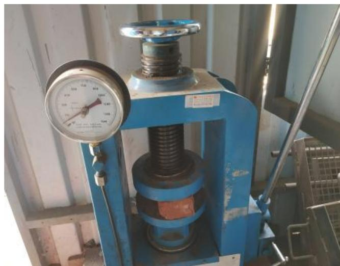
Fig-2: Compression Testing Machine (CTM)
