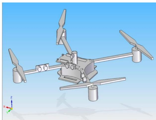
**View of the assembled drone and bird repeller system**
