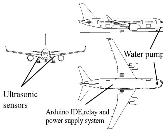
Location of the bird repeller system on an aircraft
