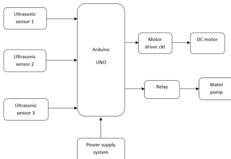
Block diagram of bird repeller system
