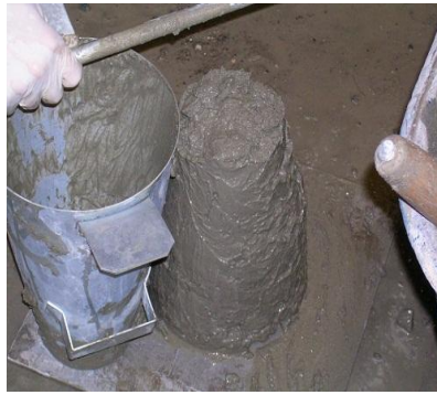
Figure 5.1: Slump Cone Test
