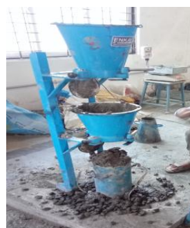
Figure 5.2: Compaction Factor test
