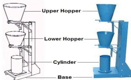
Compaction Factor Test on Concrete
