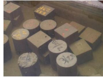
Fig: Curing of specimens
