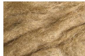
**Fig. No 4: Jute fibre**
