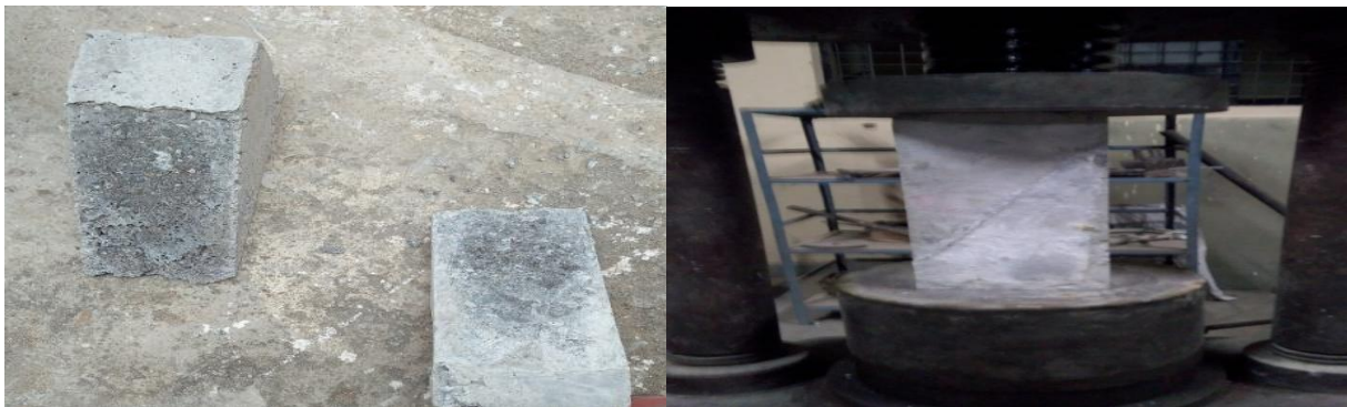
Fig. 2 Slant shear test specimens
