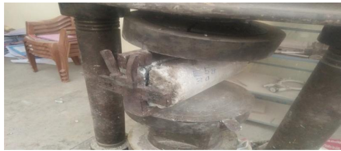
Fig.4 Failure specimen of split tensile test
