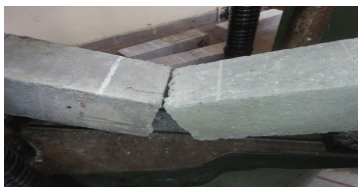
Fig.19 Failure specimen of flexural strength test
