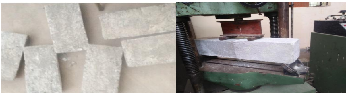
Fig. 3 Flexural strength test specimens
