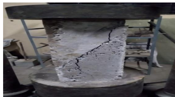
Fig. 12 Failure specimen of slant shear test
