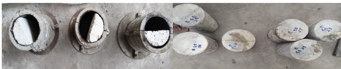
Fig. 1 Split tensile test specimens
