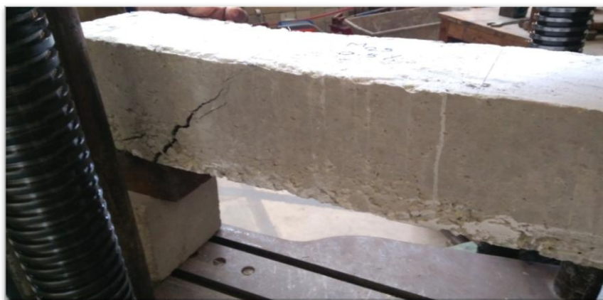
Fig 9. Shear mode of failure
