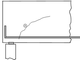
**Fig.1.2. Inclined Shear cracks**
