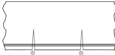
**Fig.1.1 Flexural cracks**
