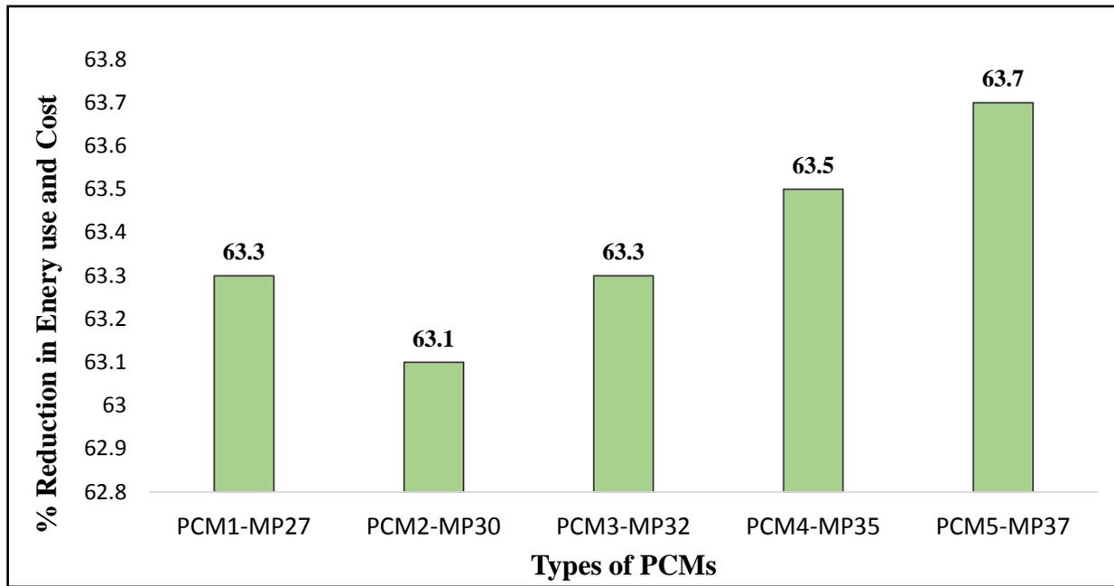
Figure 3 - Percentage Reduction in Energy Consumption in Different Models
