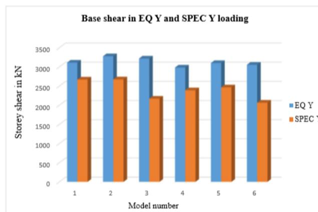
Fig 14: Graph showing Base shear values of all the Models
