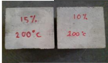
Figure 1.1: The concrete containing 10% and 15% fly ash after exposed to 200°
