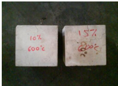
Figure 1.3: The concrete containing 10% and 15% fly ash after exposed to 600°C
