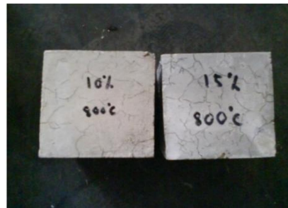
Figure 1.4: The concrete containing 15% 10% fly ash after exposed to 800°C
