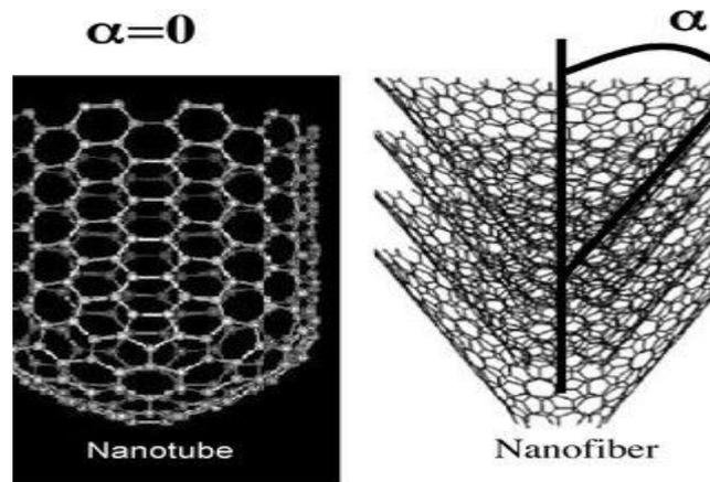
Fig3: Carbon Nano tube & Carbon Nano fiber [Source: Quoc Ngo et al. (2007)]
