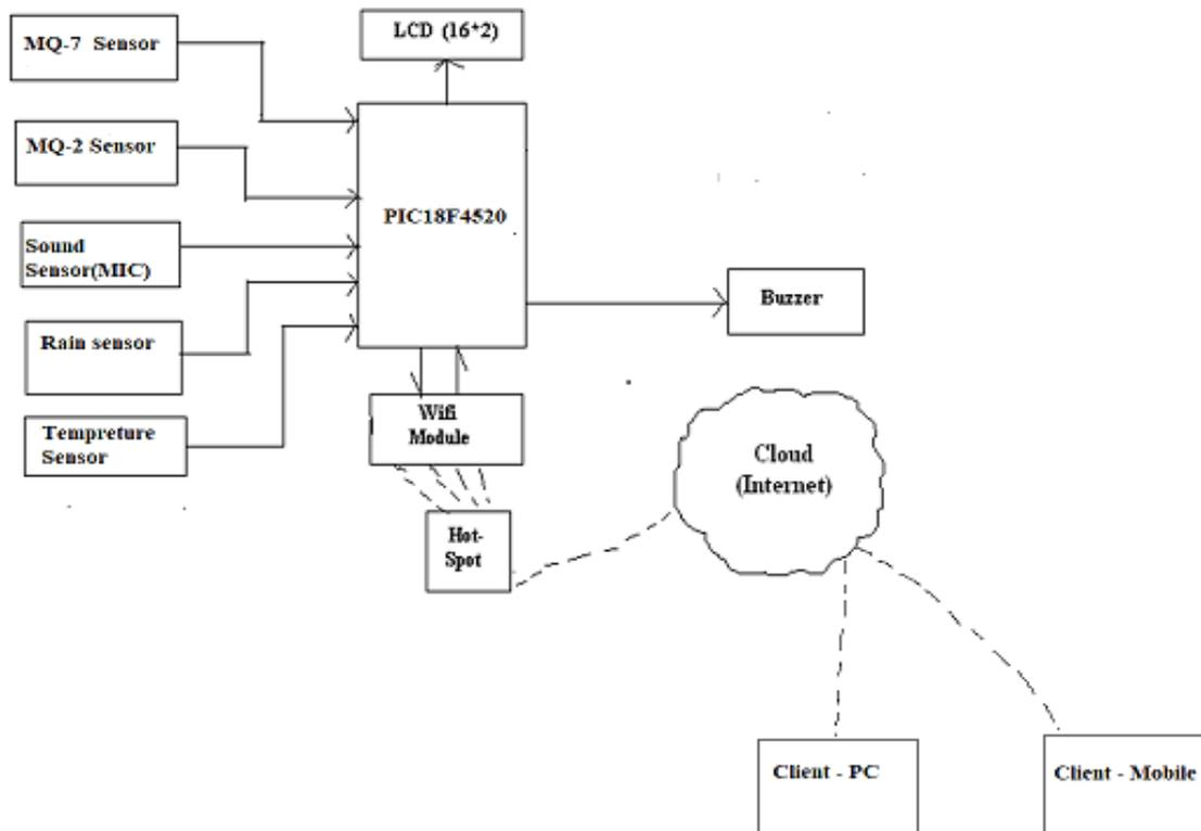
fig.1 Block Diagram
