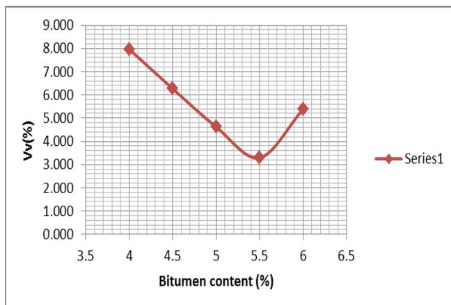
Fig. 10 Variation in Volume of Voids with Bitumen Content
