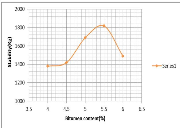
Fig. 14 Variation in Stability with Bitumen Content
