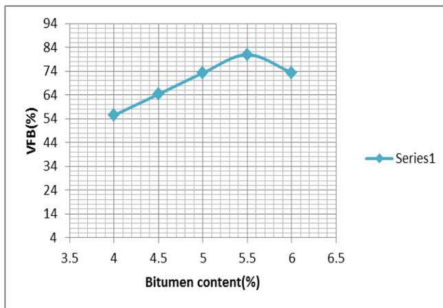
Fig. 11 Variation in Volume filled by Bitumen with Bitumen Content
