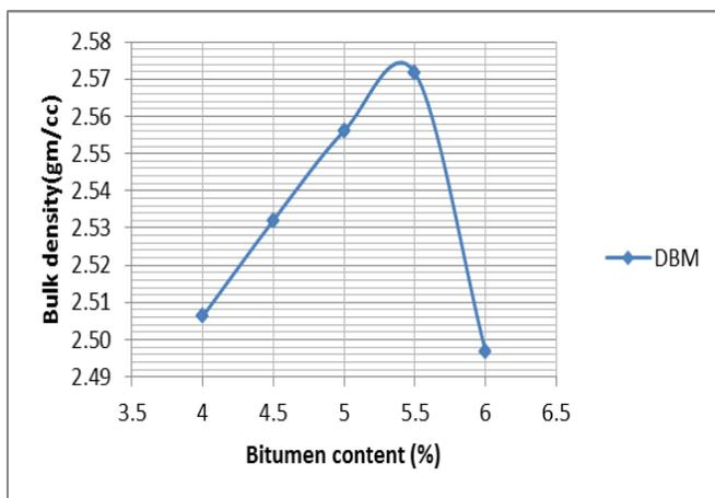
Fig. 8 Variation in Bulk Density with Bitumen Content
