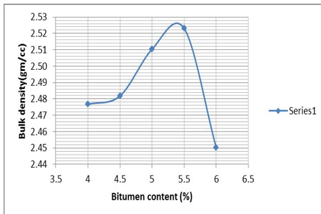
Fig. 13 Variation in Bulk Density with Bitumen Content
