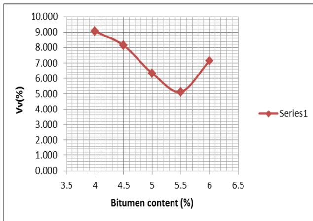
Fig. 15 Variation in Volume of Voids with Bitumen Content
