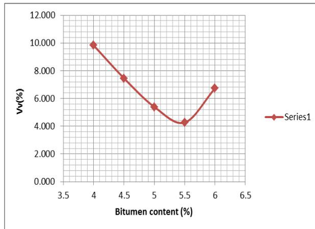
Fig. 5 Variation in Volume of Voids with Bitumen Content
