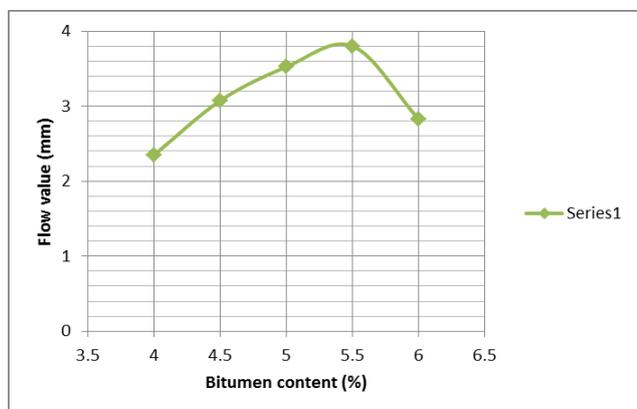
Fig. 2 Variation in Flow Value with Bitumen Content
