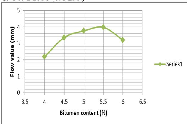
Fig. 12 Variation in Flow Value with Bitumen Content
