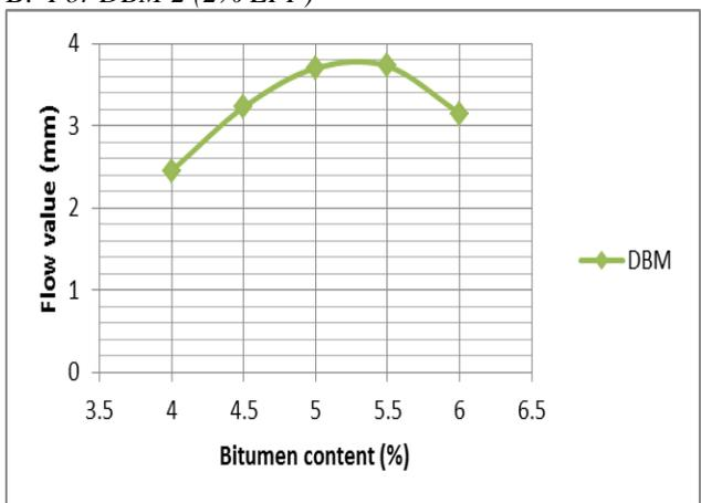
Fig. 7 Variation in Flow Value with Bitumen Content
