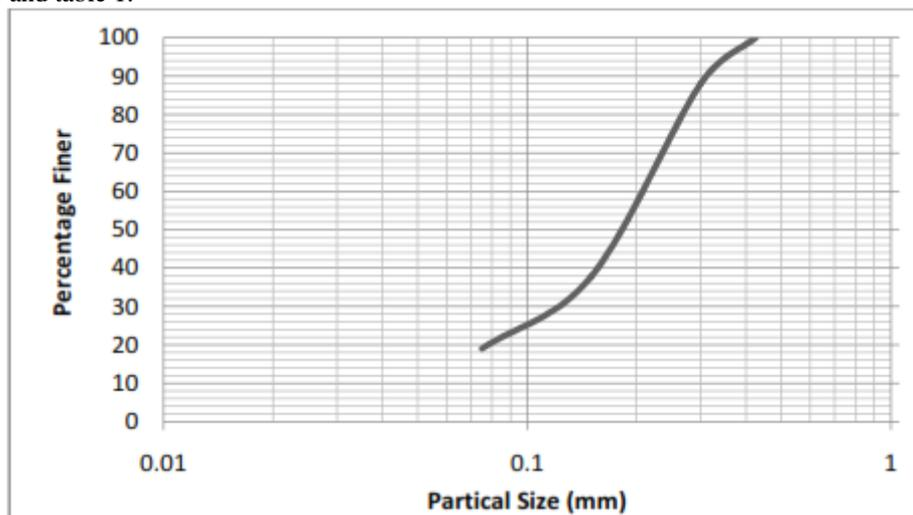
*Fig. 1 Grain size analysis distribution curve of E-waste plastic powder*
