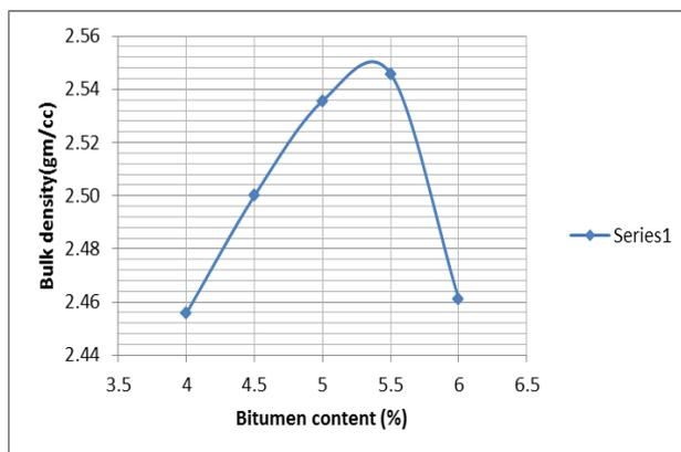
Fig. 3 Variation in Bulk Density with Bitumen Content
