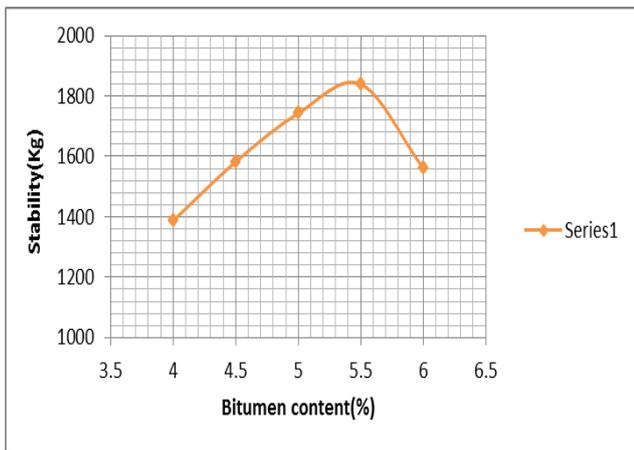
Fig. 4 Variation in Stability with Bitumen Content
