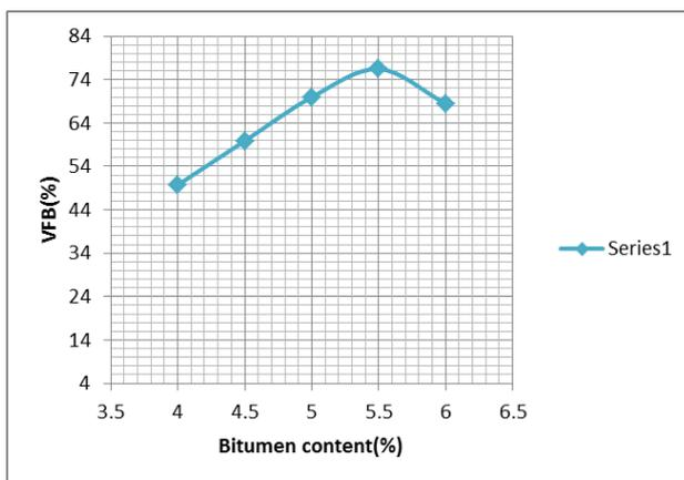
Fig. 6 Variation in Volume filled by Bitumen with Bitumen Content
