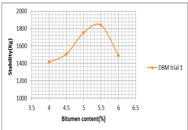
Fig. 9 Variation in Stability with Bitumen Content
