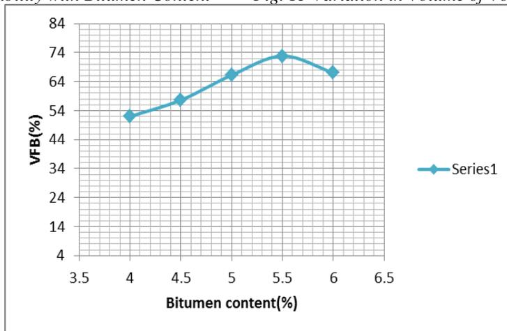
Fig. 16 Variation in Volume filled by Bitumen with Bitumen Content
