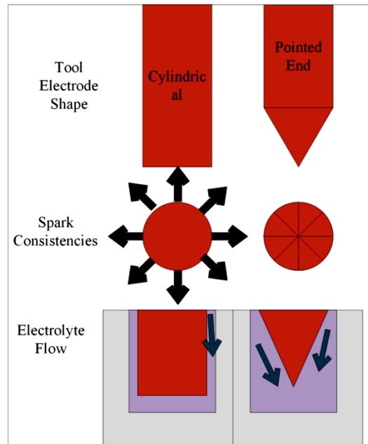
Fig.6. Flow of electrolytes and Spark consistencies in different shapes of tool (Rajput et al. 2019).
