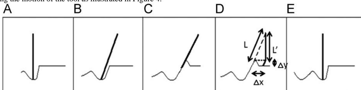
Fig. 4. Tool stick and Jump phenomena (Jana et al. 2012).
