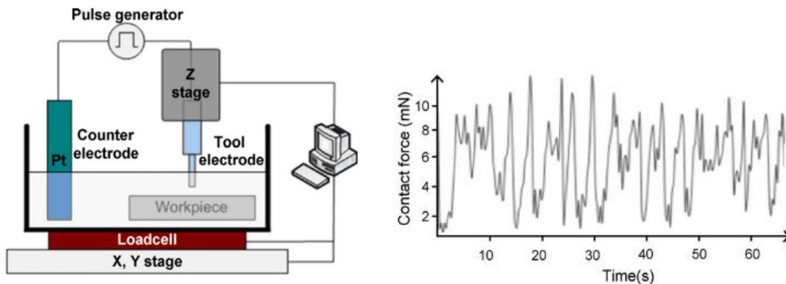
Fig. 3. (a) Schematic Diagram; (b) Load cell signal (Cao et al. 2009).
