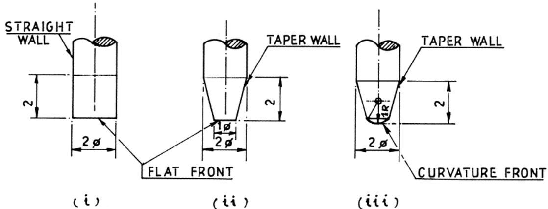
Fig. 5. Different tool shapes of the tip (Bhattacharya et al. 1999).
