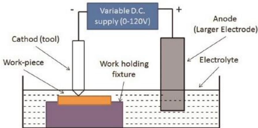
Figure 1 Schematic diagram of ECDM.
