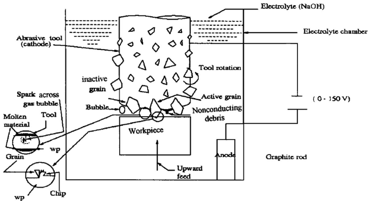
Fig. 3. Machining mechanism with abrasive cutting tools (Jain et al. 2002).
