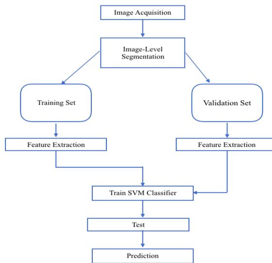
Fig 3: Flow diagram for image detection
