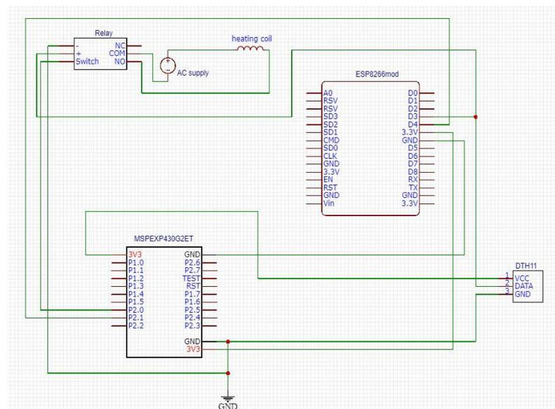
Fig2: pin diagram
