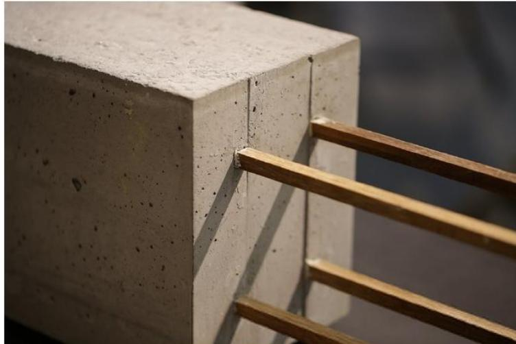
*Fig. 2: Bamboo Reinforced bars*
