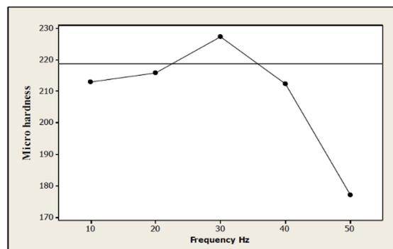
**Fig 2 Frequency vs micro hardness**
