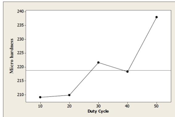
**Fig 1 micro hardness vs duty cycle**
