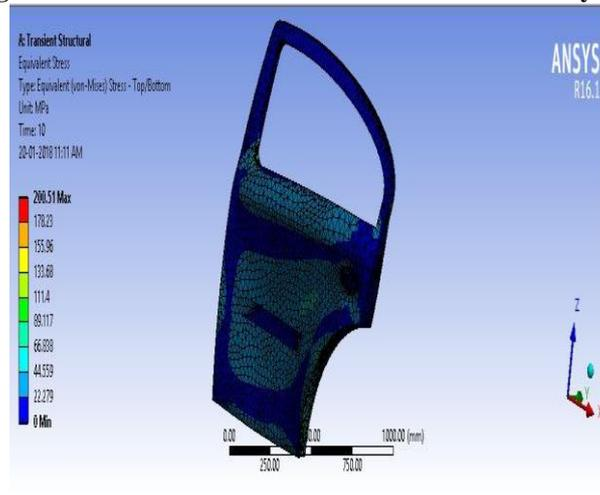
**(Fig-9 Von Mises Stress Distribution of S-Glass)**
