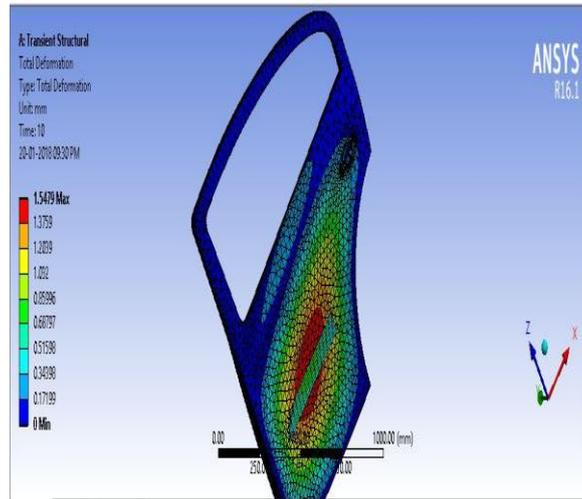
**(Fig-14 Total Deformation on Aluminum Alloy - C)**
