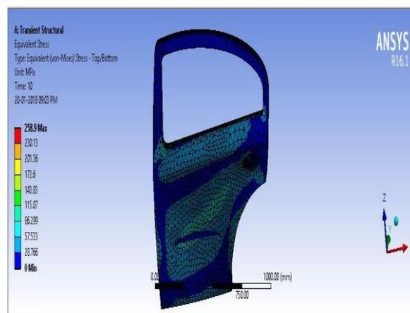
**(Fig-18 Von Mises Stress Distribution on E-Glass Epoxy-C)**
