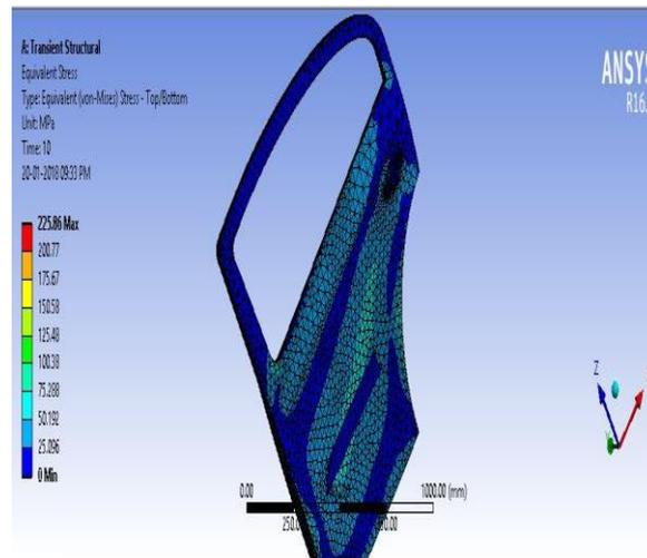
**(Fig-17 Von Mises Stress Distribution on Aluminum Alloy-C)**
