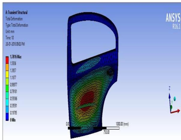
**(Fig-15 Total Deformation of e-glass - c)**
