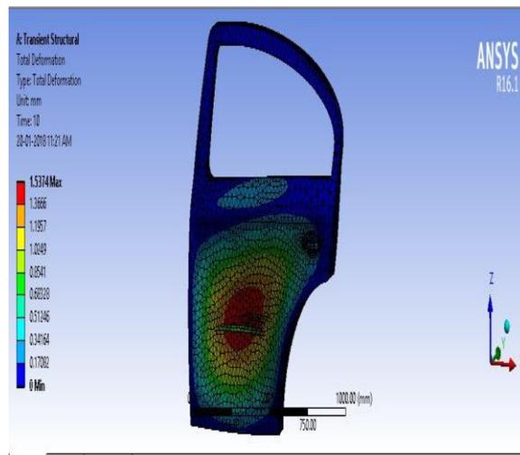
**(Fig-12 Total Deformation of e-glass -box)**
