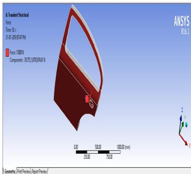
**(Fig-6: load acting on outer body)**
