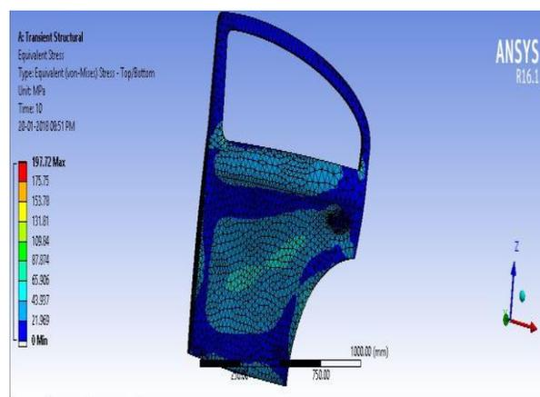
**(Fig-19 Von Mises Stress Distribution on S-Glass Epoxy-C)**
