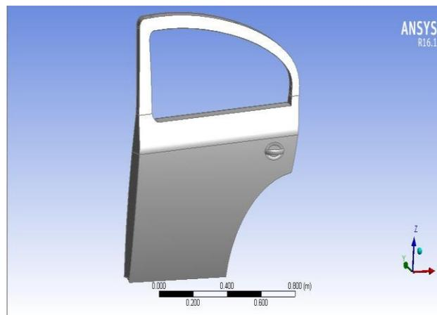
**(Fig-4: Imported model in ANSYS Workbench)**
