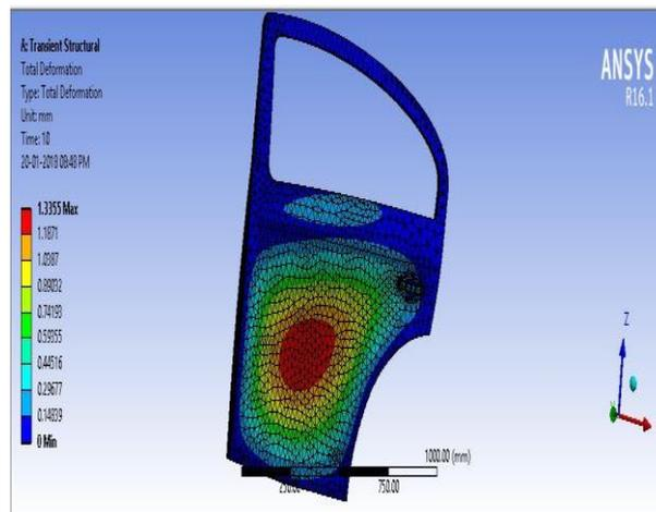
**(Fig-16 total deformation of s-glass-c)**
