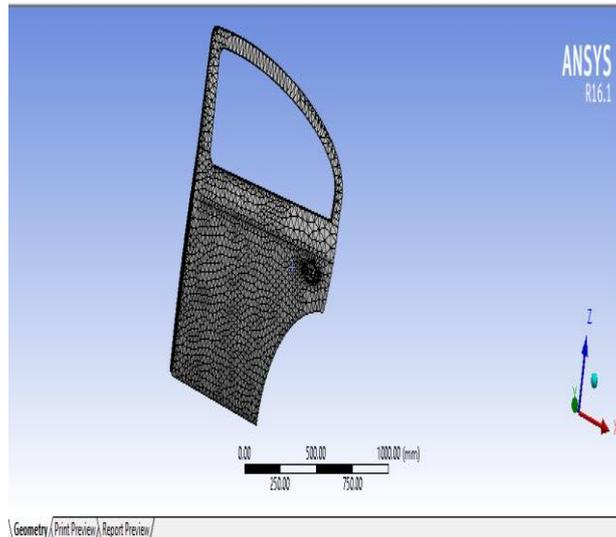
**(Fig-5: Meshed model of Car door)**
