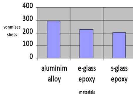
**(Fig-20 Bar Chart of Von Mises Stress observed in MPa box section)**
