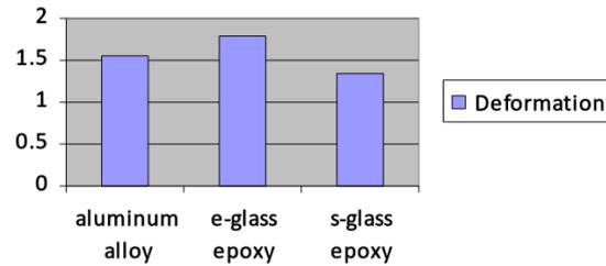
**(Fig-22 bar Chart of Deformation In mm-C sec)**
