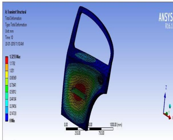
**(Fig-13 Total Deformation on S-Glass-Box)**
