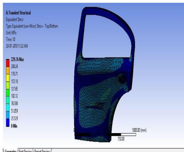
**(Fig-10 Von Mises Stress Distribution of E-Glass)**
