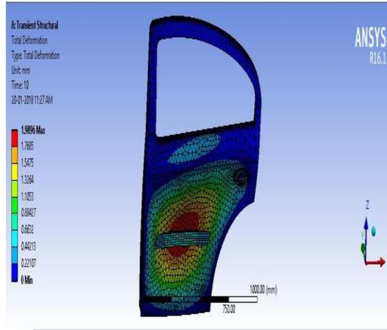
**(Fig-11 Total Deformation on Aluminum Alloy-Box)**
