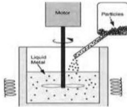
**Fig. 3.1** Stirring of composite melt with ceramic particles to minimize settling of the particles during processing
