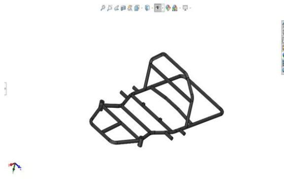
Fig.3 Isometric view of chassis
