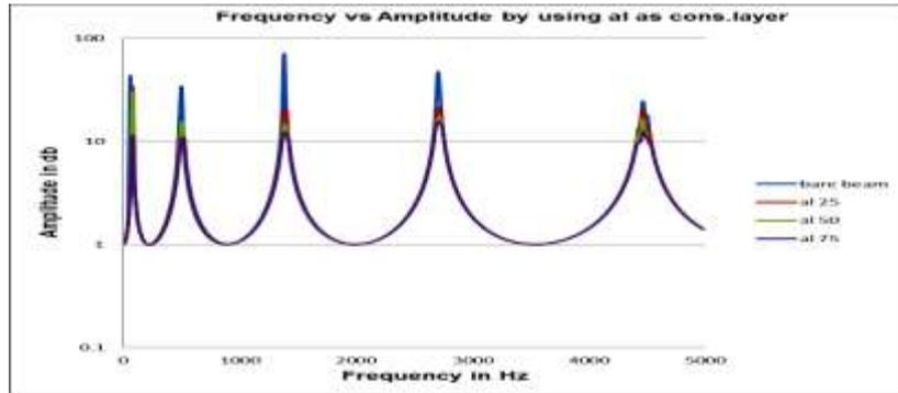
Fig - Harmonic analysis with Aluminium as constraining layer and butyl rubber as core
