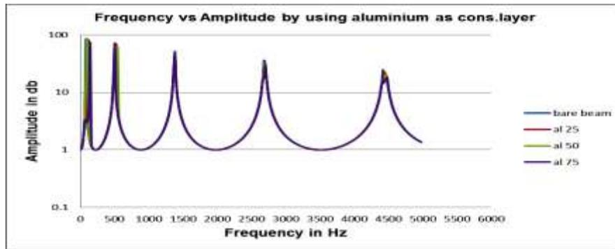
Fig - Harmonic analysis with aluminium as constraining layer and DYAD606 as core
