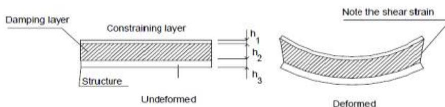
Fig Deformation of constrained layer.
