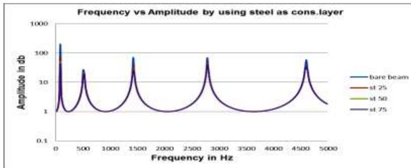
Fig - Harmonic analysis with steel as constraining layer and butyl rubber as core
