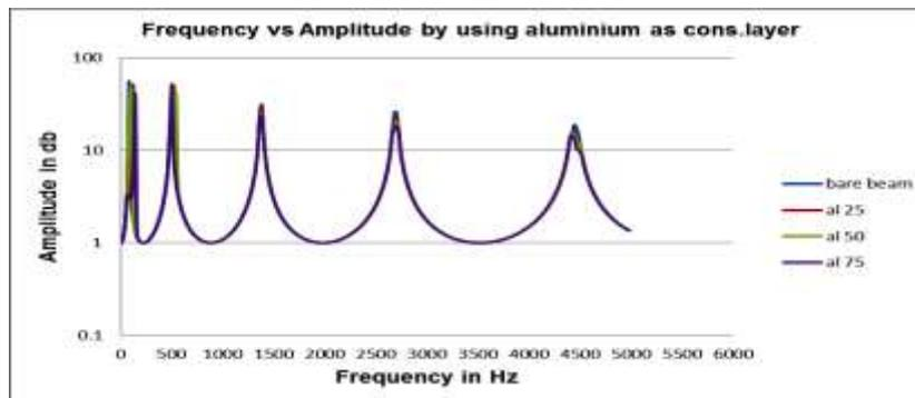
Fig - Harmonic analysis with aluminium as constraining layer and silicone rubber as core
