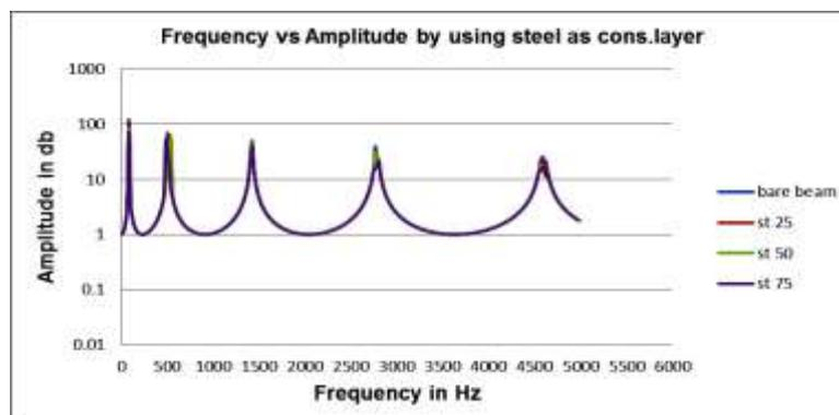
Fig - Harmonic analysis with steel as constraining layer and silicone rubber as core
