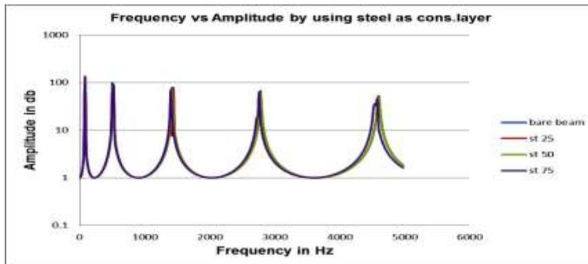
Fig - Harmonic analysis with steel as constraining layer and DYAD606 as core
