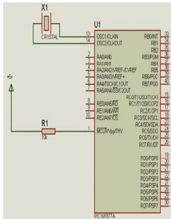
Figure 10. PIC16F877A circuit.
