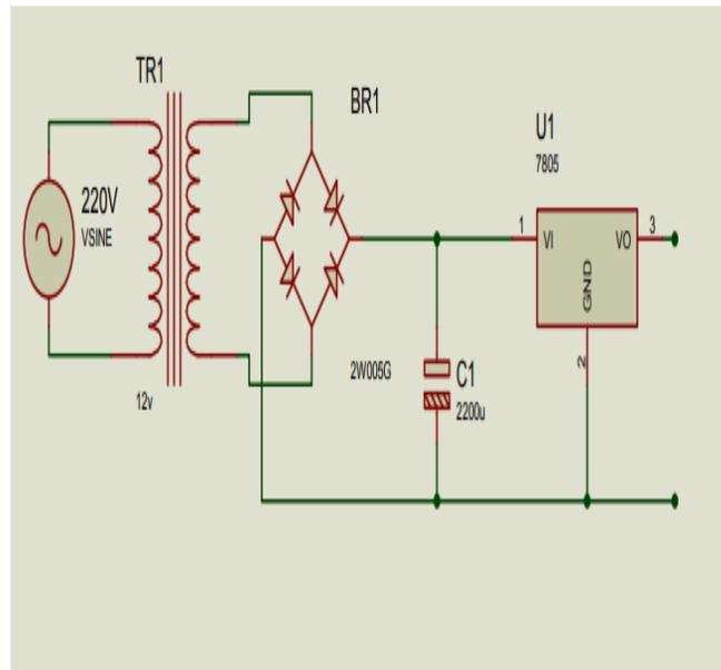
Figure 5. Powersupplycircuit.
