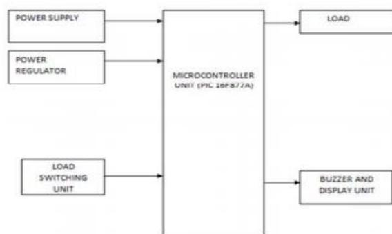
*Figure 1. Block diagram of Microcontroller load sharing and control system.*
