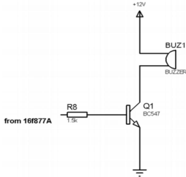
**Figure 8.** Alarming circuit.
