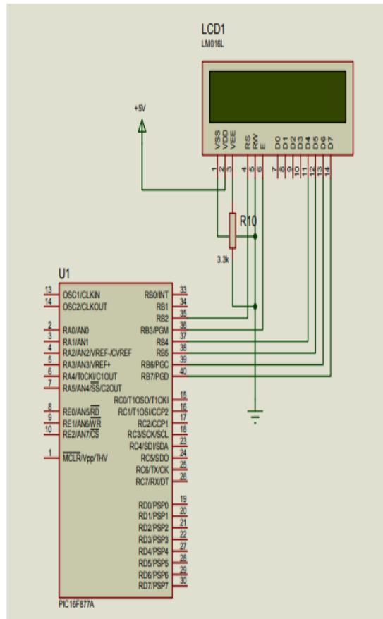
Figure 9. LCD interfaced to PIC16F877A.
