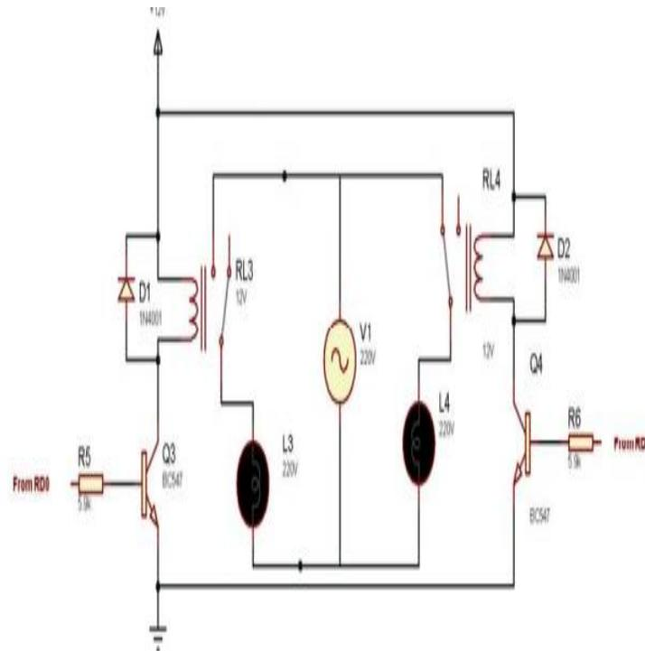
Figure 7. Load control circuit.
