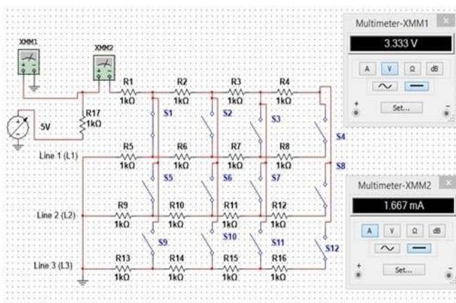
Fig. 2. Simulation model of resistors and switches using NI Multisim
