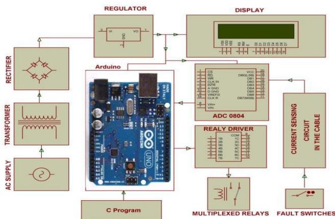
Fig. 1. Underground cable fault distance locator block diagram
