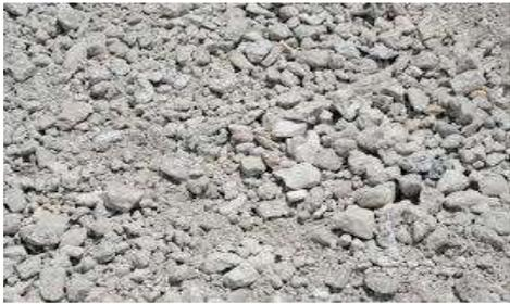
**Figure 3 Recycled Aggregate Concrete(RAC)**
