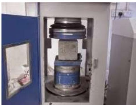
**Figure 6 Compressive test**
