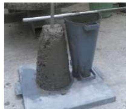
**Figure 7 Workability test**
