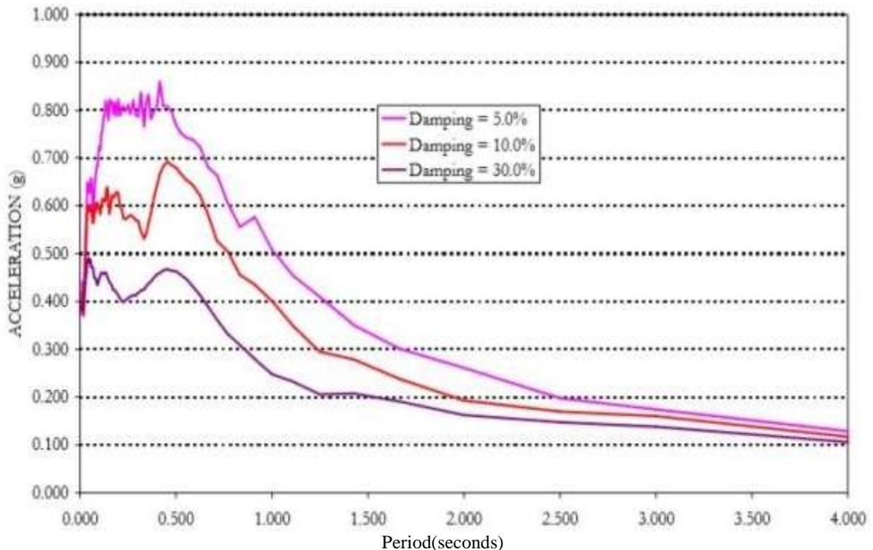
**Figure 4: Effect of damping on Acceleration**
