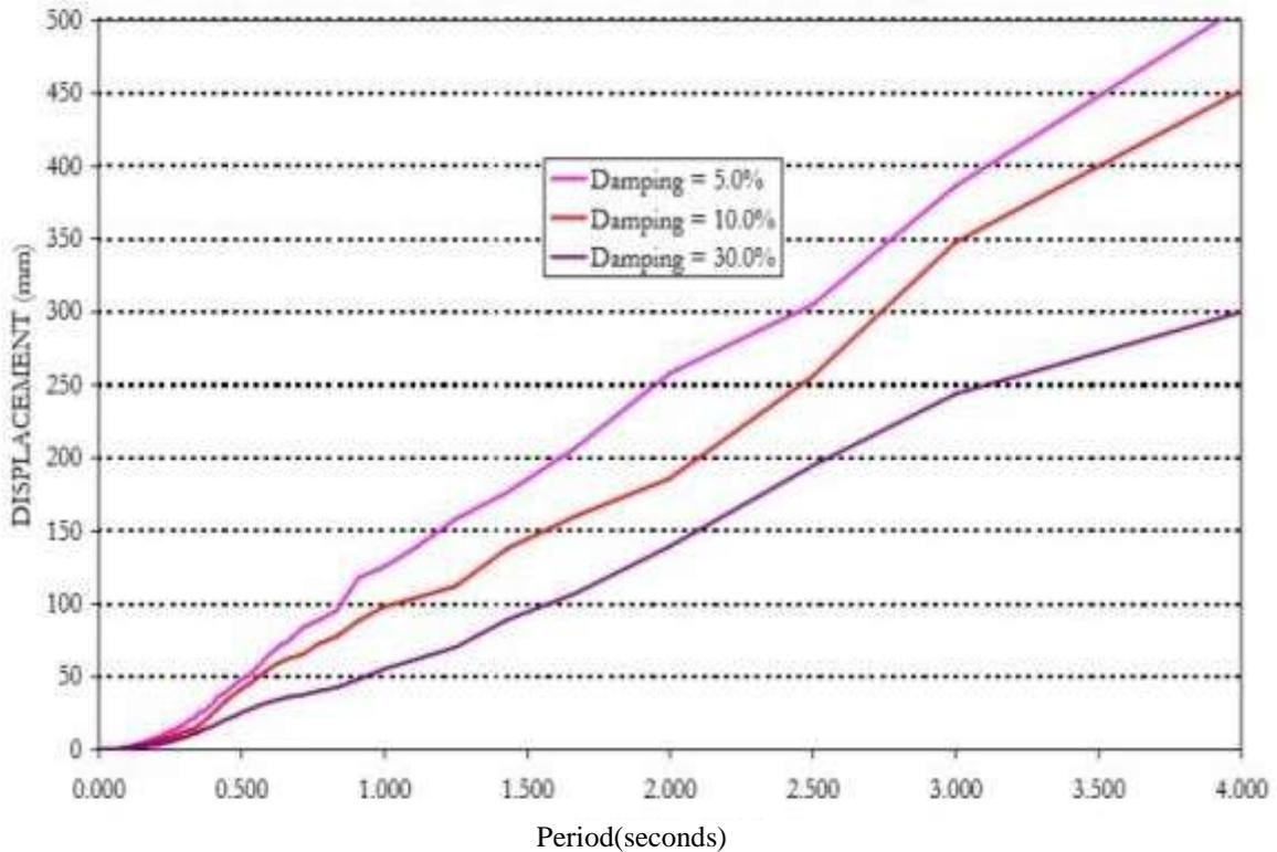
**Figure 3: Effect of damping on Displacement**
