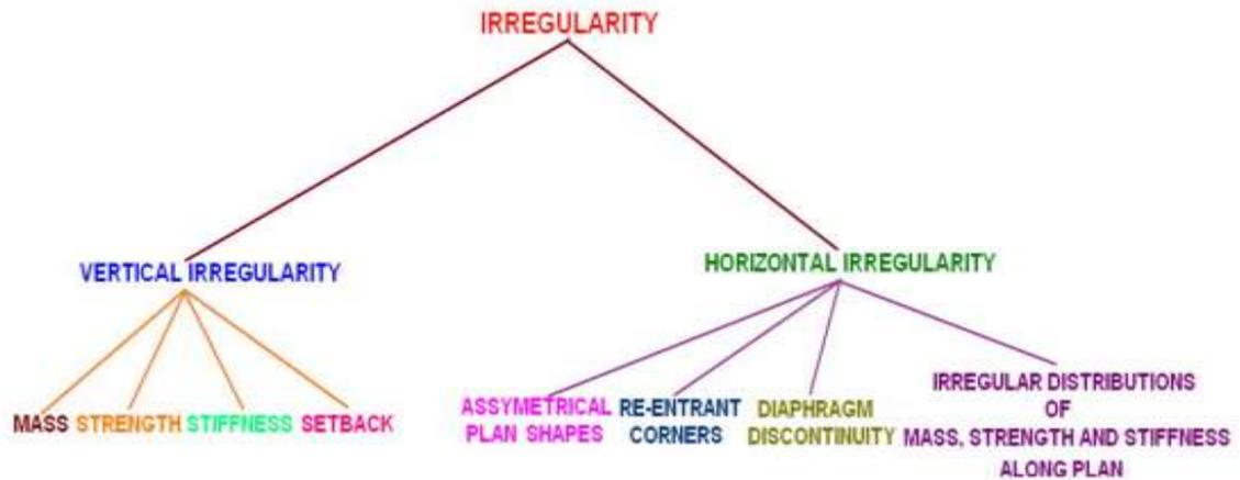
Figure 1.1 Classification of different types of structural irregularities
