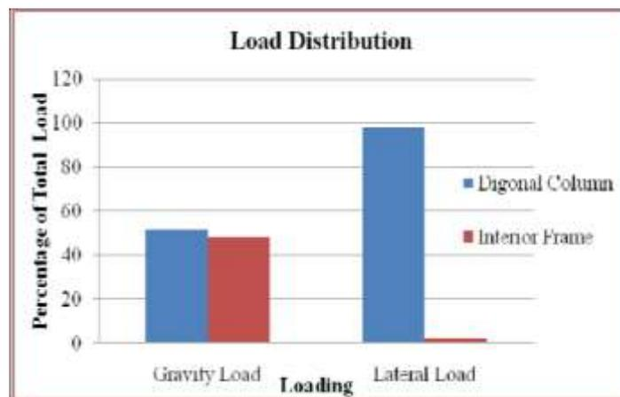
Figure 6: Load distribution in exterior and interior frame <sup>[7]</sup>
