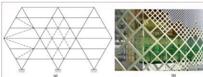
Figure 4: Secondary Bracing System in diagrid [5]
