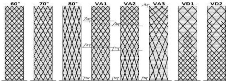
Figure 2: Different geometry patterns of diagrid structure [4]
