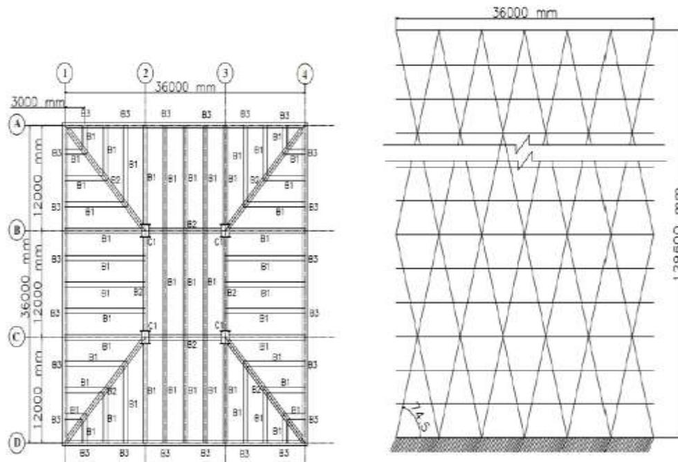
Figure 5: Typical Floor Plan Elevation of 36 Storey Buildings <sup>[7]</sup>
