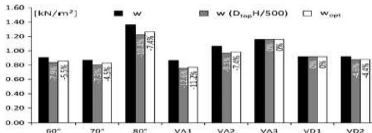
Figure 3: Unit steel weight of diagrid patterns [4]
