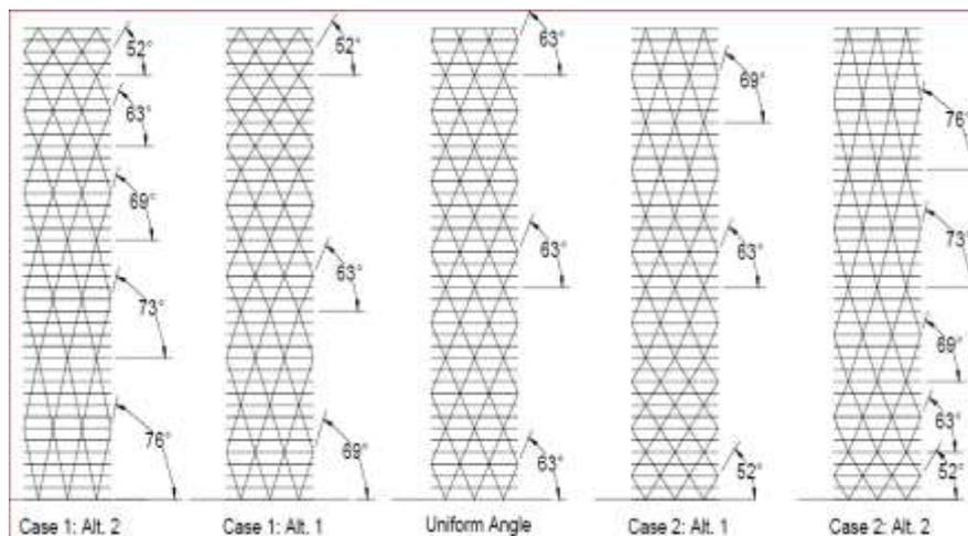
Figure 1: Variously configured 40-storey diagrids (H/B = 4.3) <sup>[3]</sup>
