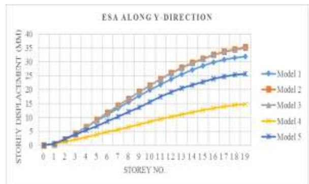
**Figure 4 Equivalent Static Analysis of storey displacement in Y-direction**
