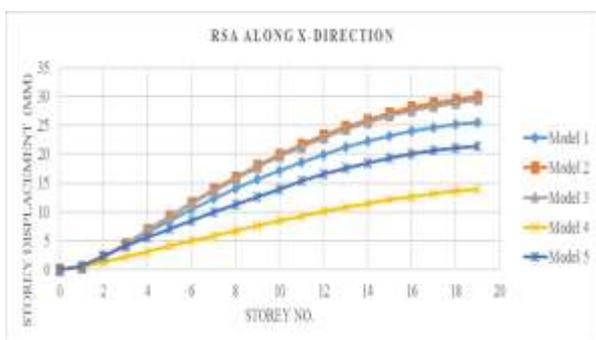
**Figure 5 Response Spectrum Analysis of storey displacement along X-direction**
