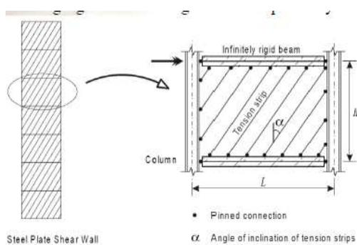
**Fig. 1: Strip Model Representation of a SPSW**
