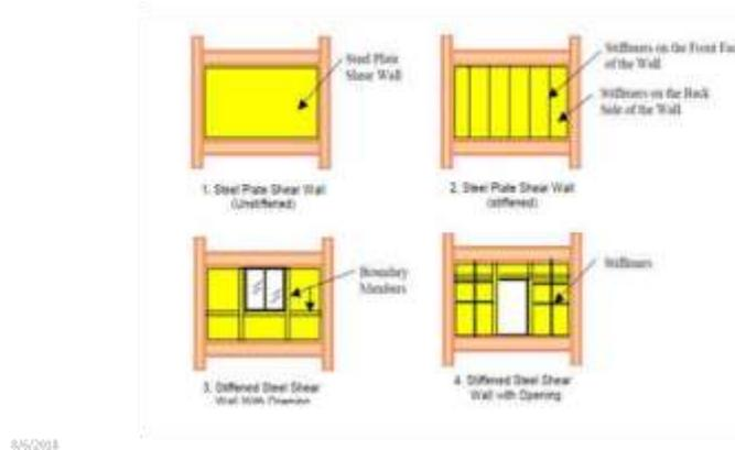
**Fig.1: Types of Steel plate Shear Wall**
