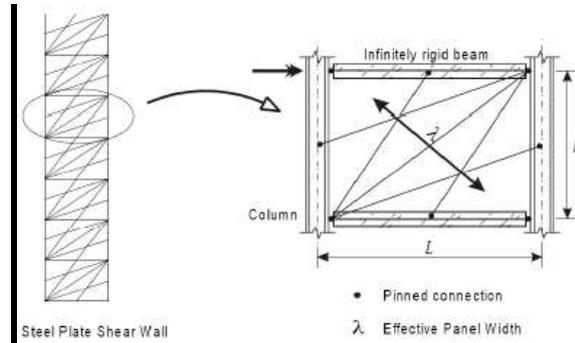
**Fig. 2: Multi-angle strip model of a SPSW**
