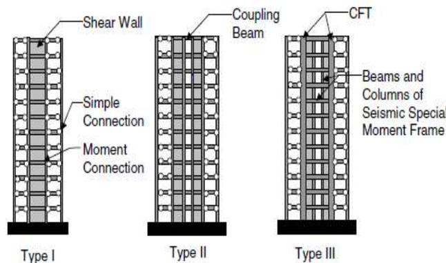
**Figure 1. Three common types of steel shear wall systems.**
