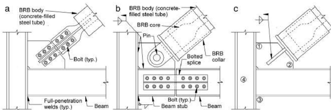
Figure 4: a) continuous beam bolted brace b) split beam pinned brace c) continuous beam welded brace [19]
