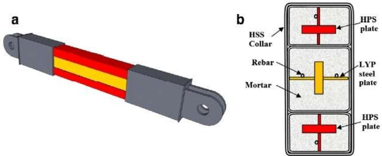
Figure 5: Hybrid Buckling-Restrained Brace [2]
