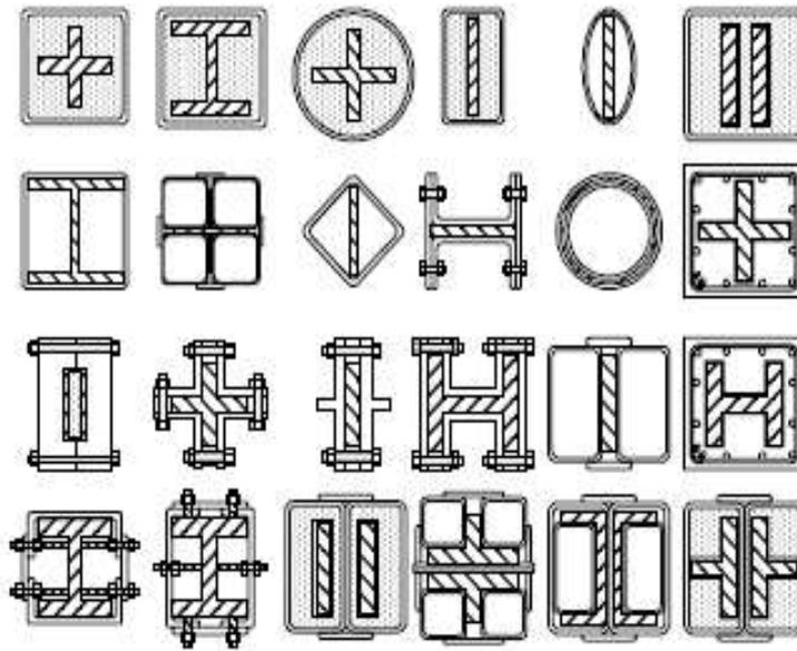
*Figure 1: Typical Cross-Section of BRBs [17]*
