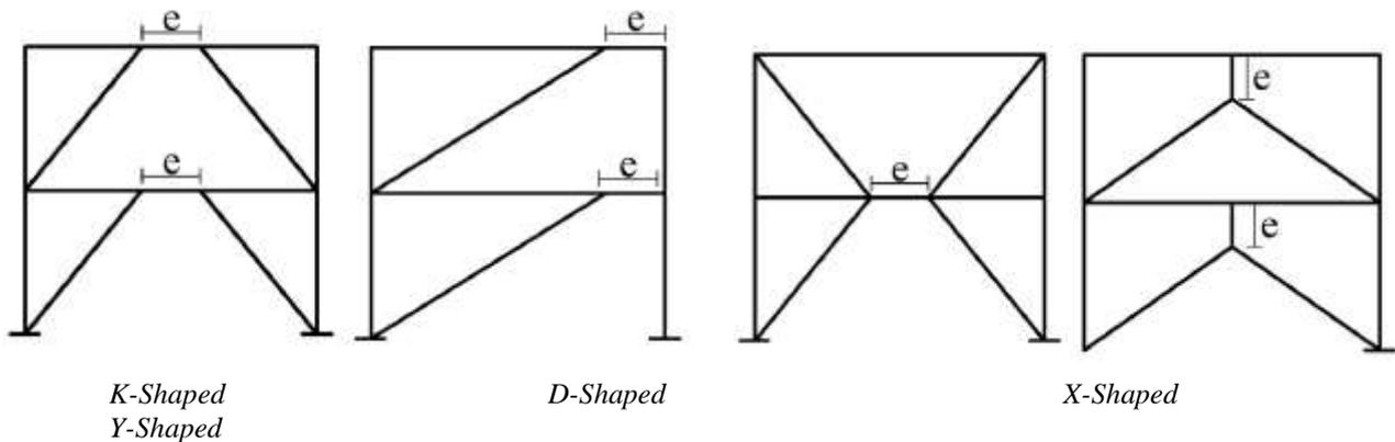
*Figure 7: Typical Eccentrically Braced Frames [19]*
