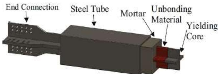
*Figure 2: Scheme of arrangement of all Material [12]*
