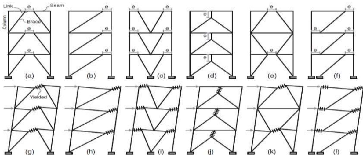
Figure 6: EBF configurations and their corresponding plastic mechanisms. [3]
