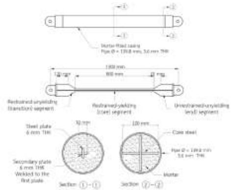
Figure 3b: Detailing of BRKB
