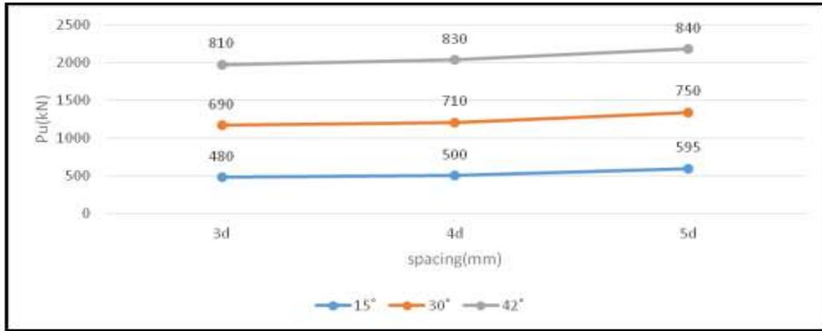
Fig. 2.-Ultimate Load Vs Spacing Between Piles for 4x4 Piles <sup>[1]</sup>
