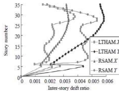
Figure 16. Inter-story drift ratio under MCE
