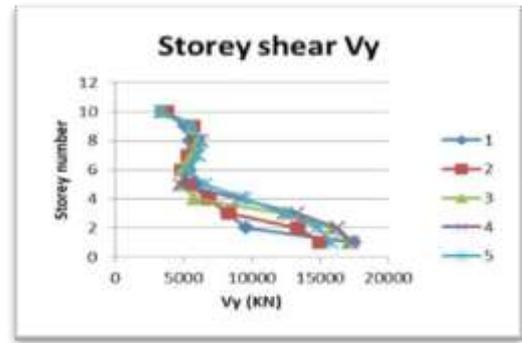
Figure 5. Storey shear distribution in Y direction
