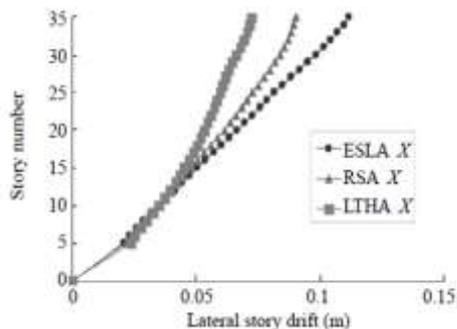
Figure 11. Later story drift in the X-direction under frequent earthquakes
