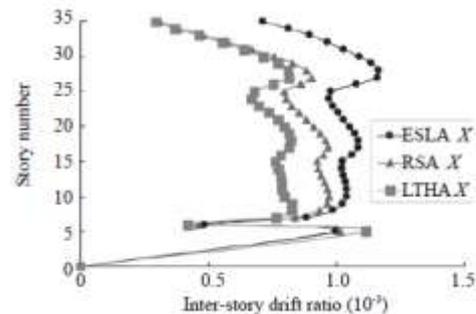
Figure 12. Inter-story drift ratio under frequent earthquakes
