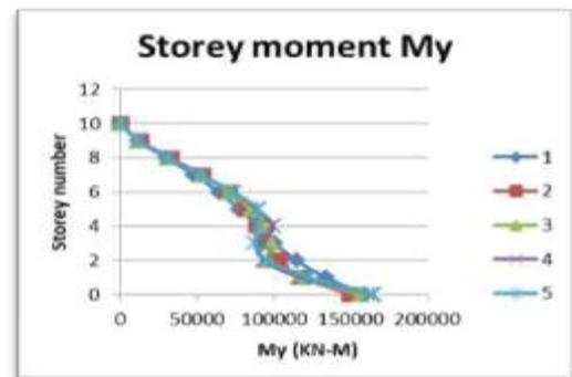
Figure 7. Storey moment distribution in Y direction
