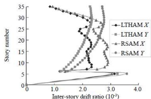
Figure 14. Inter-story drift ratio under DBE
