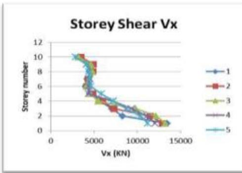
Figure 4. Storey shear distribution in X direction
