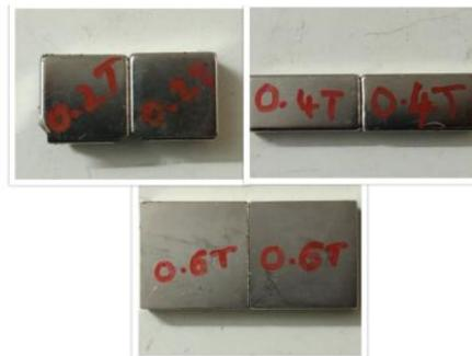
*FIG.2:-Neodymium magnets with different magnetic power(0.2T,0.4T,0.6T)*
