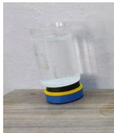
*Fig. 2 Beaker placed over the magnets for magnetizing the water*
