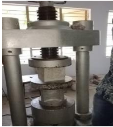
Figure.2a. Picture showing testing of cubes under 100 T Compressive testing machine
