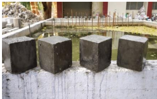
Figure.4 Cubes cast with magnetic water and cured with normal water.
