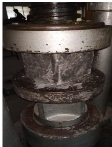
Figure.5 Failure of test specimen.
