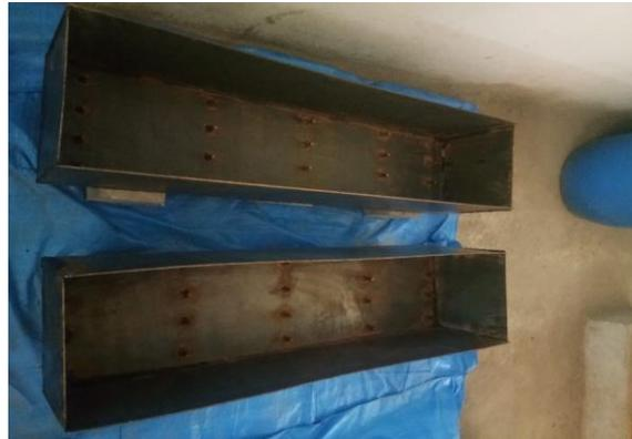
Fig.1 Specimens welded with shear studs
