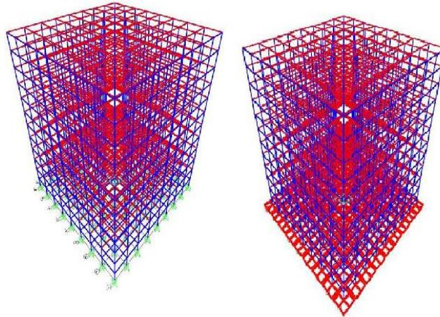
Fig:6 Building Models with fixed base and with SSI case (Martin et al (2017) ).
