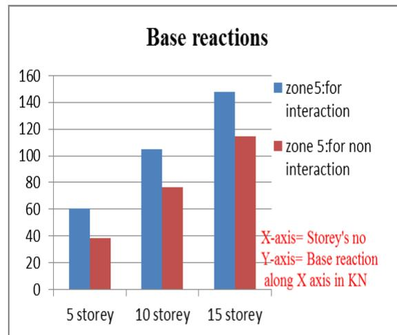
Fig. Base reactions for fixed base condition and SSI condition Zubair et al (2016)
