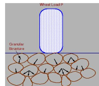
1. *Conventional flexible pavements* are layered systems with high quality expensive materials are placed in the top where stresses are high, and low quality cheap materials are placed in lower layers.
