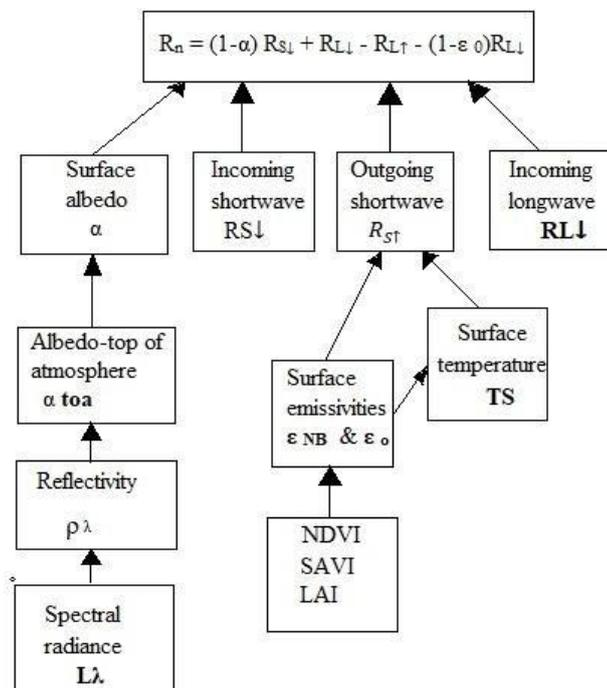
Figure 3.1 Flow chart of Computation of Net Surface Radiation
