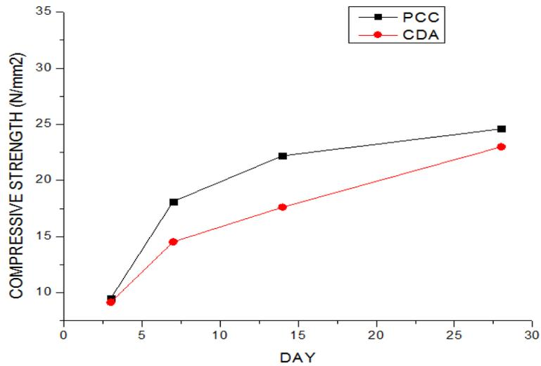
GRAPH SHOWING COMPRESSIVE STRENGTH OF PLAIN CONCRETE AND 20% COW DUNG ASH
