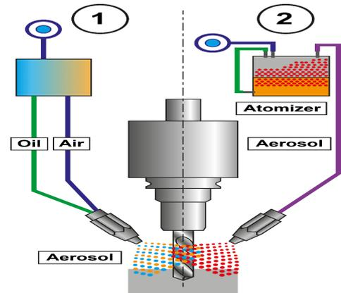
Fig.3. Internal Delivery Systems [2]
