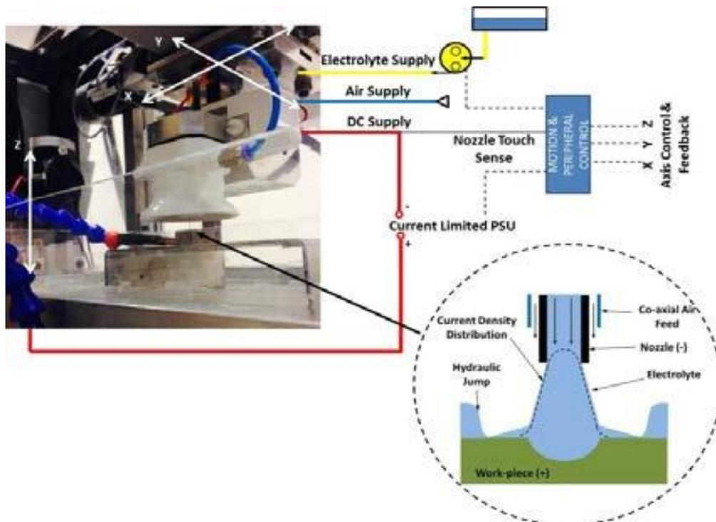
Figure 3: Schematic of Electrochemical Jet Machining apparatus and process [25]
