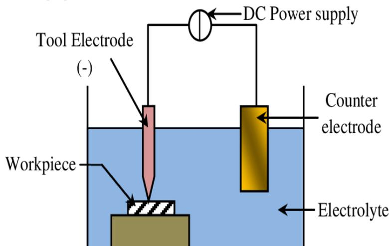
Figure 4: Electrochemical discharge machining [27]
