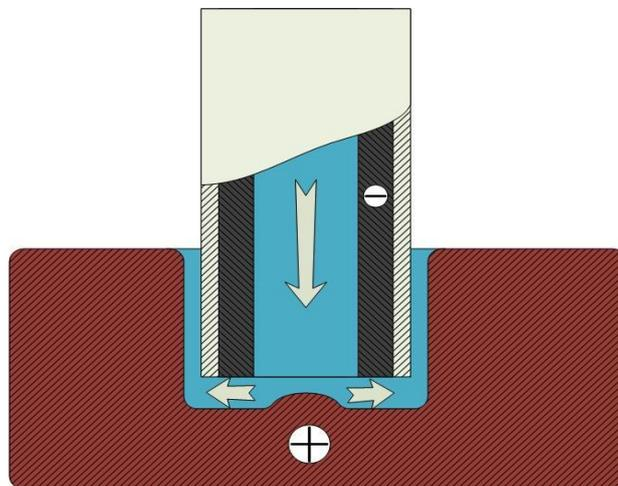
*Figure 2: Processing principle of Electro Chemical Drilling [20]*
