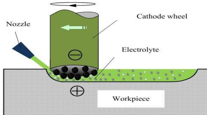
Figure 5: Schematic diagram of electrochemical grinding [28]
