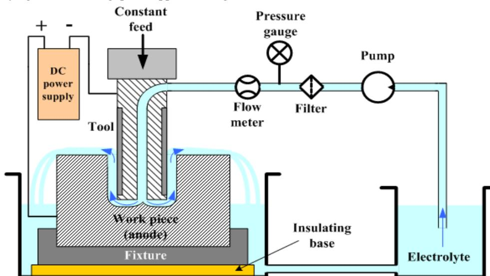
Figure 1: Schematic diagram of ECM
