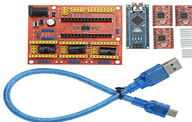
Fig. 4 CNC Shield V4.0
