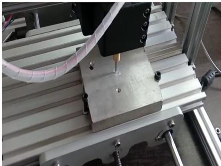
Fig. 9 Engraving "S" on Aluminum
