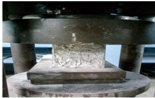
Fig 8: Testing and failure pattern of cube
